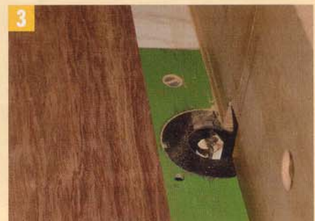
Fit the router table with a 19mm straight cutting bit...
