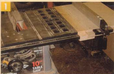
To cope with panel cutting, I extended the size of my saw table with a home-made extension table
