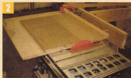
To get a square end, place one edge of the panel against the fence and run it through the saw. Note that the guard is removed for clarity
