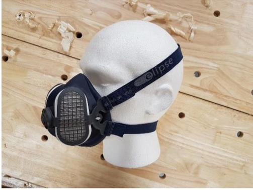
When creating particularly fine dust, which is basically when sanding, the use of a face mask is also a good idea. They can be disposable or reusable. The reusable type offer a better seal around the face and can also be used when spraying or applying a finish. They can even remove odours.
