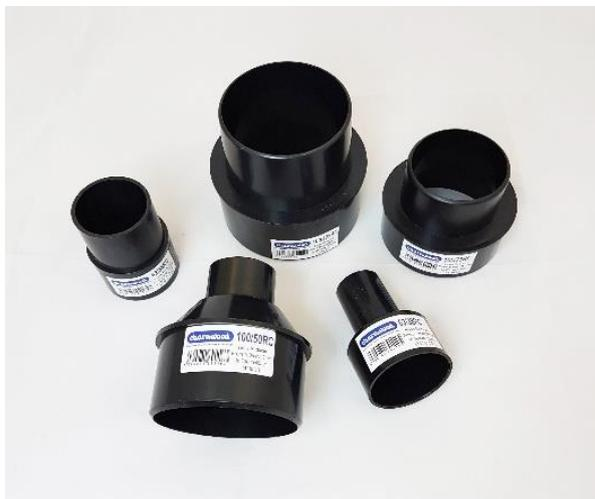
A range of Reducers are available to convert bench top machines and power tools to 100mm. They can be fitted over the outside or on the inside of the existing outlet. Carefully measure any outlets you have which are not 100mm and check the table for the best fit. If nothing seems to do the job (or the outlet is not round) there is the option of heat shrink sleeve which can be used on any outlet from 38mm to 100mm diameter.
