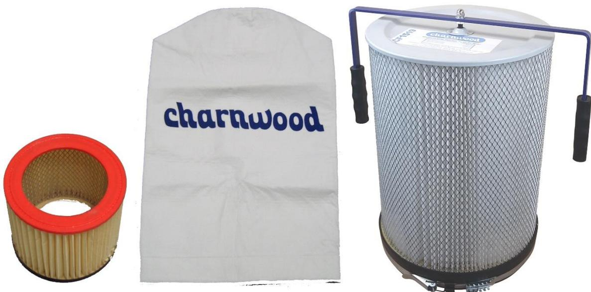
A typical hobby level high volume dust extractor will be supplied with a cloth filter, with a rating of 5 microns. That means it will filter out 99% of dust particles at 5 micron size or bigger. It will also trap some smaller particles too but to a lesser level, so at 1 micron it might only be 50%.
