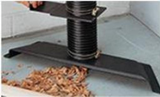
The other option is to bring the dust to the extractor by using a floor mount dust hood. The dust hood is connected to a hose branch from the extractor. Turn the extractor on and use a brush to sweep the chips into the mouth of the dust hood.
