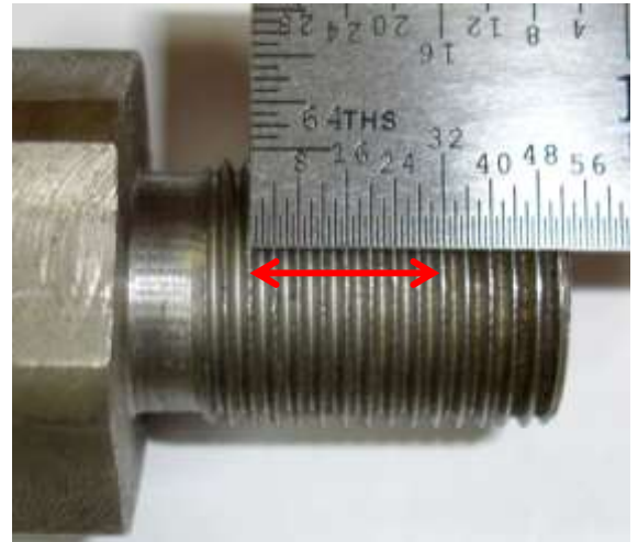
Example = 8 threads in 1/2" = 16tpi
